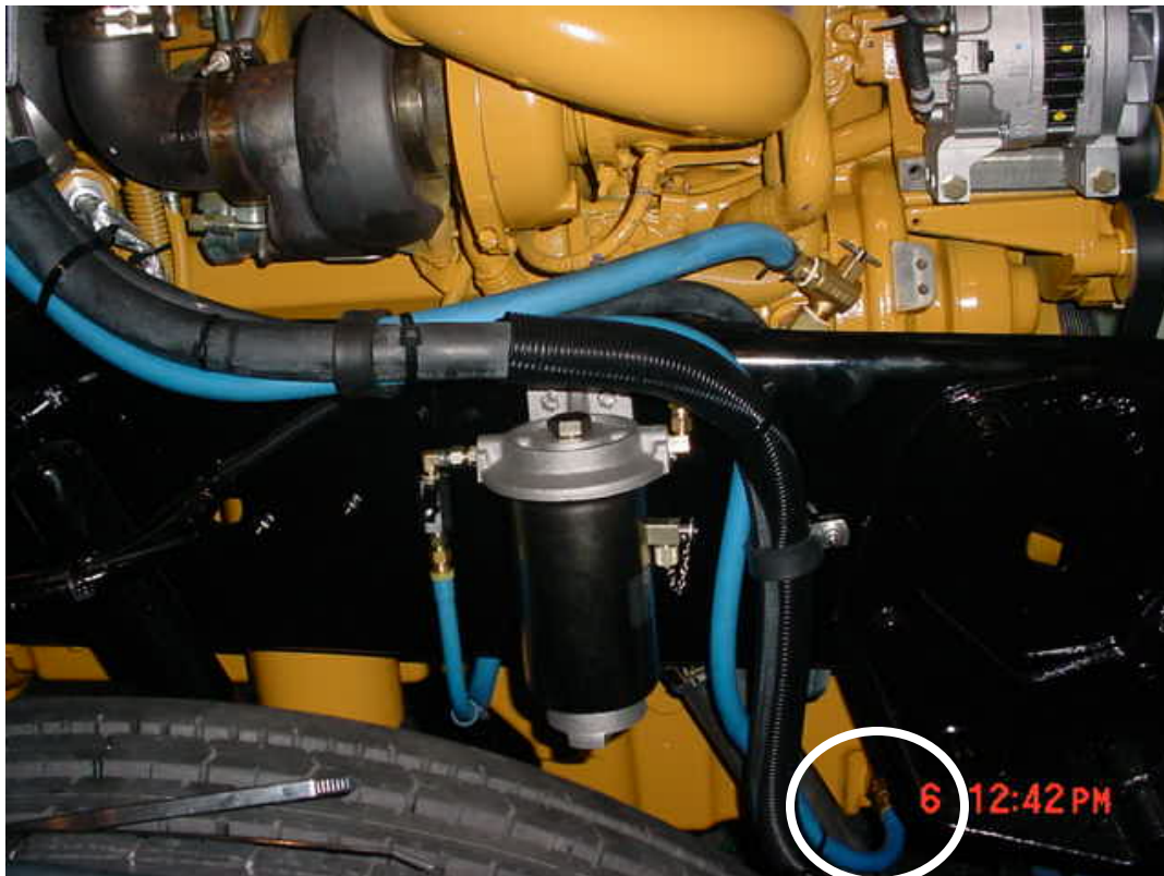
Figure 8 – Locating the Port on the Oil Pan
