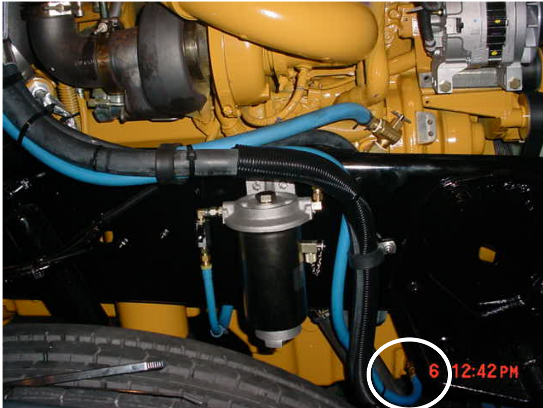
Figure 8 – Locating the Port on the Oil Pan
