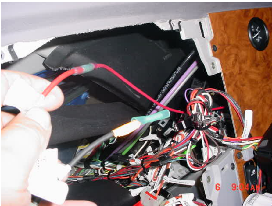
Figure 14 – Connecting the Power Lead
