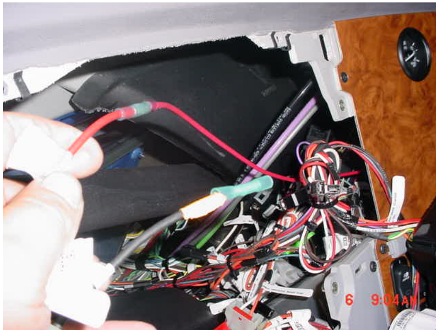
Figure 14 – Connecting the Power Lead
