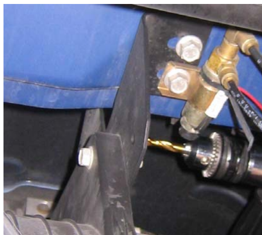
Figure 2 – Drilling the Evaporator Mounting Holes
