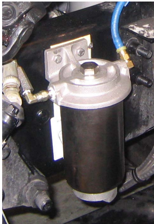
Figure 5 – Mounting the Filter to the Frame
