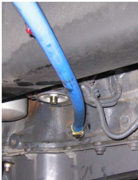
Figure 9 – Attaching the Hose to the Adaptor Fitting
