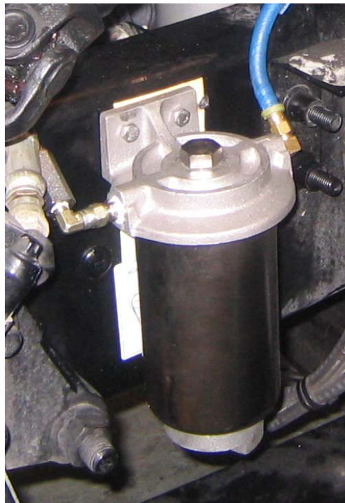
Figure 5 – Mounting the Filter to the Frame
