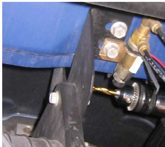
Figure 2 – Drilling the Evaporator Mounting Holes
