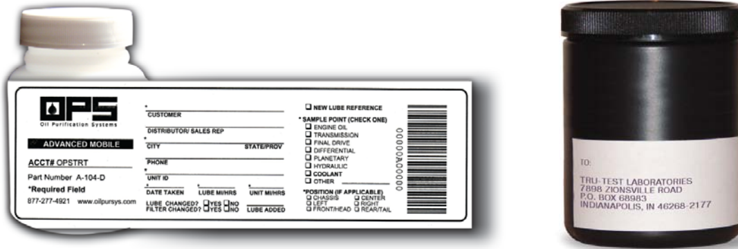
Fig. 7 – Sample bottle and shipping container. (Be sure to completely fill out the information on the label.)
