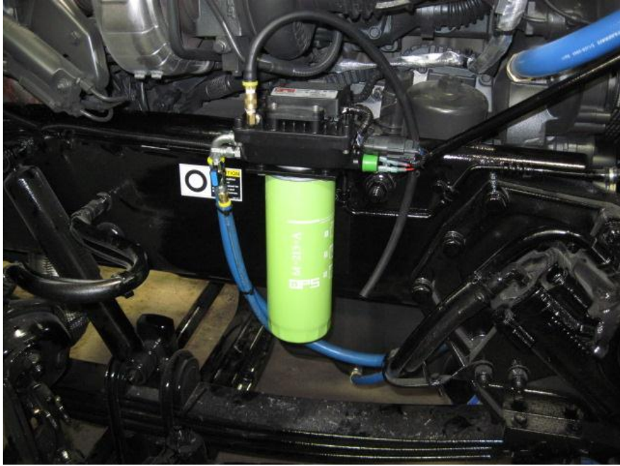
This shows the Eco-Pur mounted to the bracket and hoses attached.
