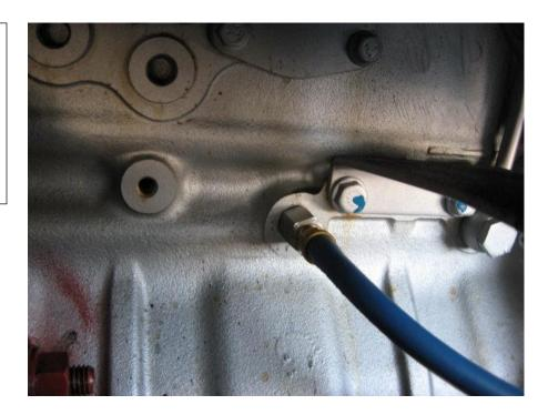
This photo shows the return hose connection on the right (passenger) side of the oil pan.
