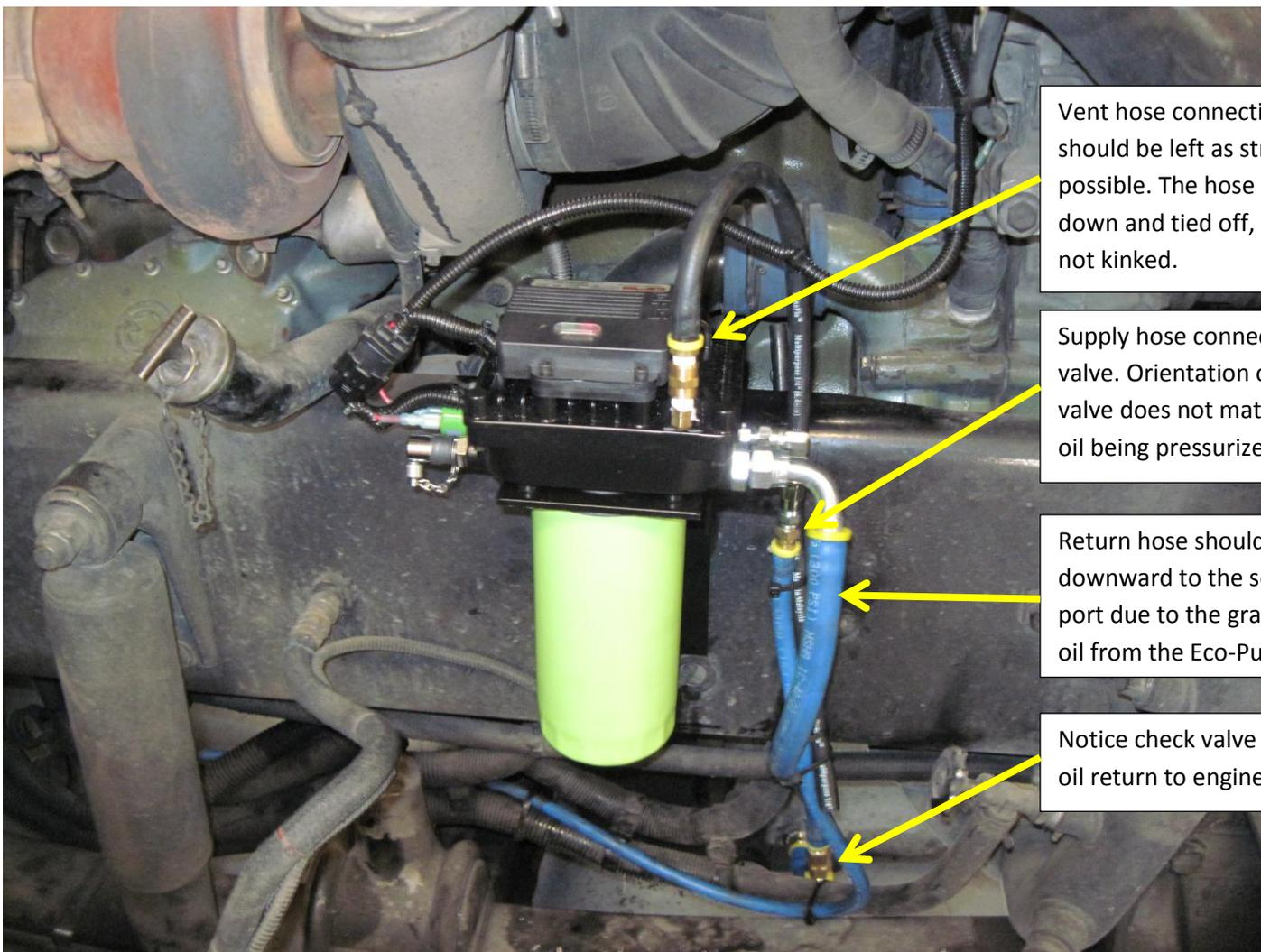
Vent hose connection. The fittings should be left as straight up as possible. The hose can be turned down and tied off, as long as it is not kinked.
